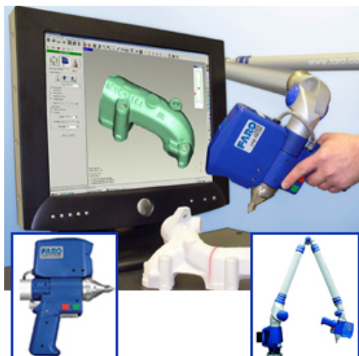
Figura 4 – Scanner laser 3D.
